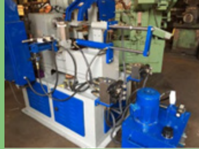
Figure 15: Special purpose drilling machine at Bharat International
