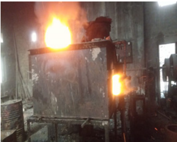
Figure 4: Conventional furnace oil fired forging furnace
