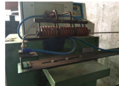
Figure 7: An induction billet heater
