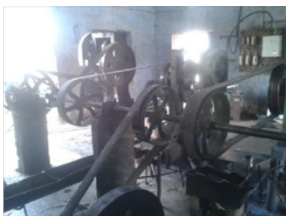
Figure 17: Common shaft with V-belt
