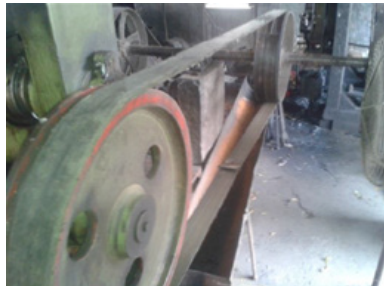
Figure 16: Common shaft with flat belt
