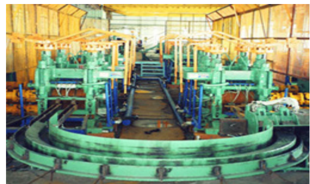
Figure 34: Repeater in steel rolling mill
