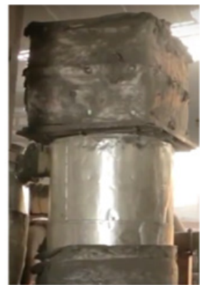
Figure 13: Radiative cum convective recuperator
