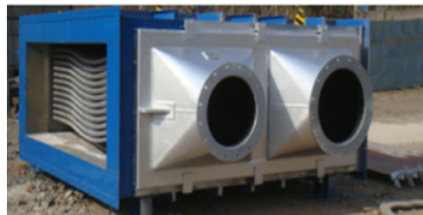
Figure 14: Cross-flow U-tube type metallic recuperator
