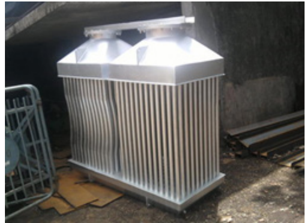
Figure 11: High efficiency metallic recuperator
