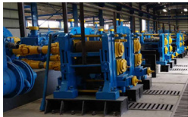
Figure 32: Universal coupling and spindles in rolling mill
