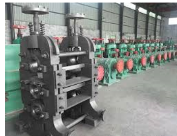
Figure 28: Roller bearing based mill stand
