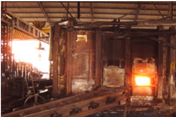
Figure 6: Conventional re-heating furnace
