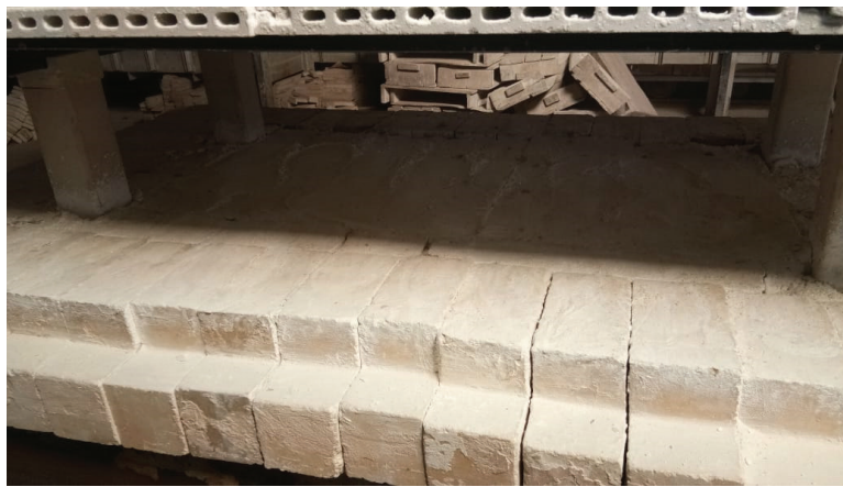
Figure 19: Existing High Thermal mass refractory in Kiln car
