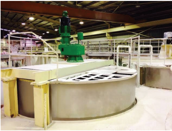
Figure 5: Slip agitation and storage
