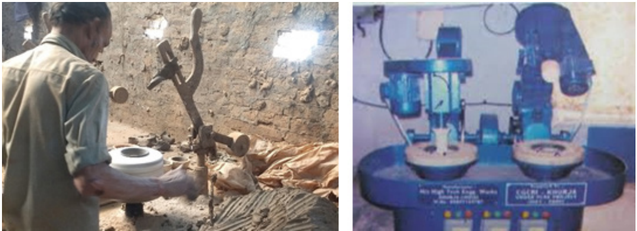
Figure 26: Manual Jigger vs automatic double roller head jigger machine
