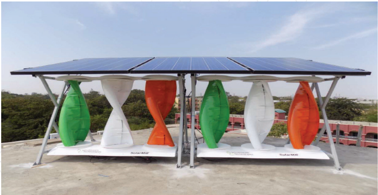
Figure 51: Solar wind hybrid system
